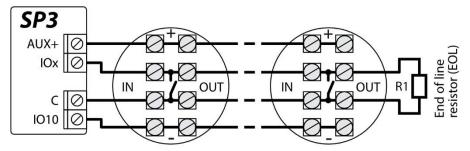
Schematic for connecting two-wire smoke detectors.
