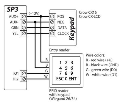
Up to 2 RFID readers can be connected to the control panel. If 2 RFID readers are connected to the control panel, no keypads can be connected.
