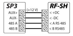
With the **RF-SH** it is possible to connect 64 wireless remote controls, 16 wireless sirens, 32 wireless sensors, 8 wireless keypads to the security system.
