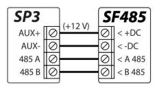
**SF485** works as secondary channel for security panel events transmission to CMS (Central Monitoring Station) or **Protegus** mobile app over the SigFox network, when primary channel fails. Events are transmitted in Contact ID format.
