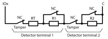
Normaly closed with End of line resistor, with tamper and wire fault recognition (3EOL)
